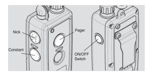
The transmitter for the **dogtrd** 2300NCP Advance single dog unit has four buttons (one on the face of the transmitter, two on the left side and one on the right side).
