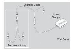
The battery charger and charging cables allow you to charge both the transmitter and receiver at the same time. The battery charger is designed for a 120-volt wall outlet. (European 230-volt AC chargers and 10-volt car charger for Lithium-Polymer batteries are also available.)
