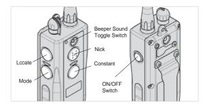
The transmitter for the **dogtra** 2500 T&B Series has five buttons.(two on the face of the transmitter, two on the left side, and one on the right side.)
